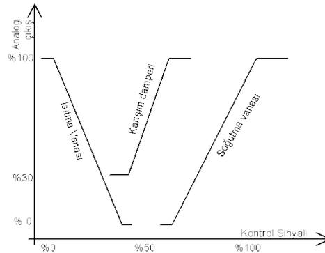
A gap of 1% should be left between control signals of sequential controlled outputs.
